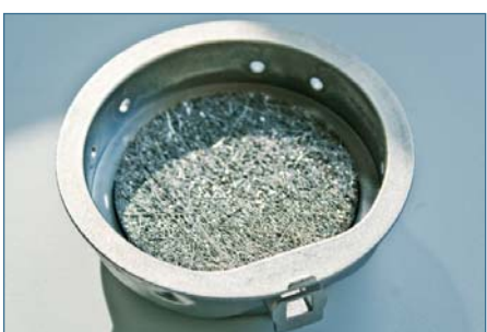
Fig. 2: Evaporation assembly with filter element for park heating system
